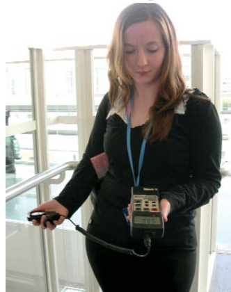
Seeing the light: Alison uses a lux meter to check out the lighting levels in the East Atrium
